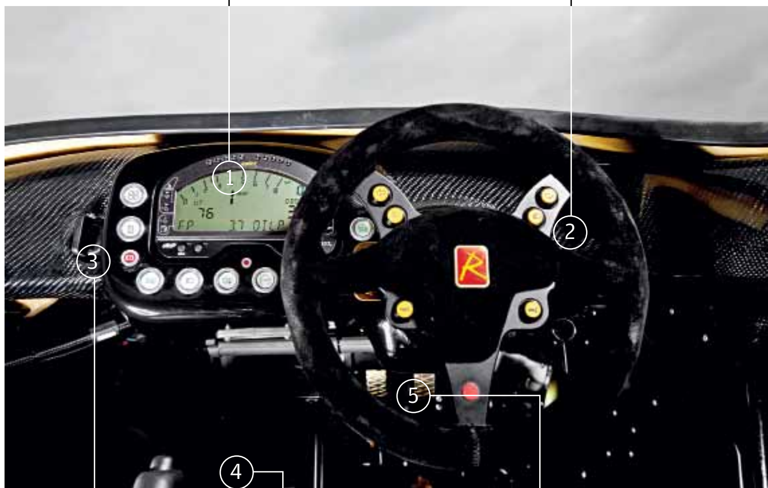
3 Fuel cut-off knob is to the left of the instruments. Turn this before you turn the ignition on, then thumb the starter button to the right of the rear foglight button.
