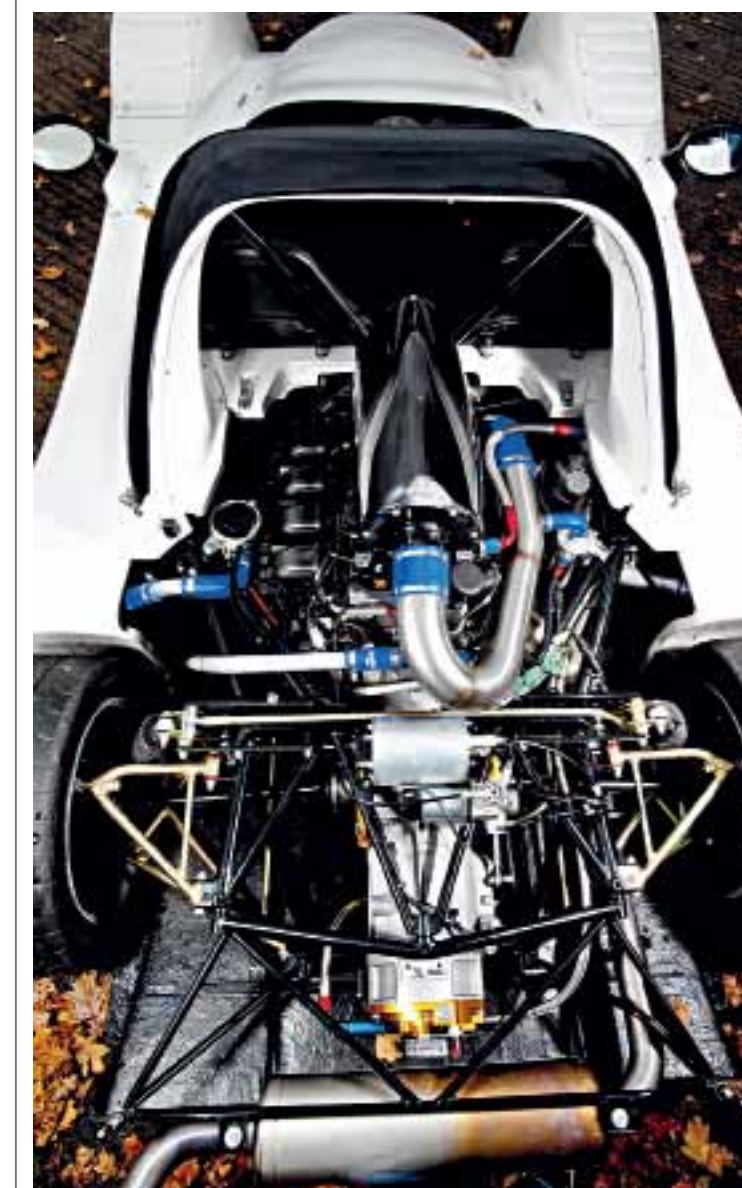
Tuned 2.0-litre Ford engine makes 245bhp; six-speed 'box and diff are by Quaife
