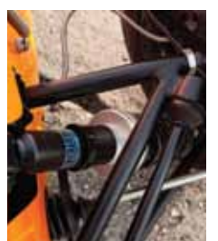
Above: Caterham's Bilstein dampers on show; set-up of the Superlight has improved since we last tried one
