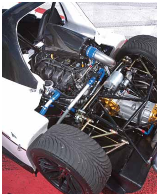
Above: Radical is powered by the turbocharged 2-litre engine from the next Focus ST. It's tuned to 300bhp here, which is more than enough
