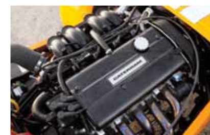
Above: Caterham Supersport has a 140bhp 1.6-litre Duratec engine mated to a five-speed manual gearbox. Below: attractive Ginetta coupe has little in the way of direct competition
