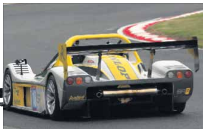
Most of the car's impressive grip comes from aerodynamics
